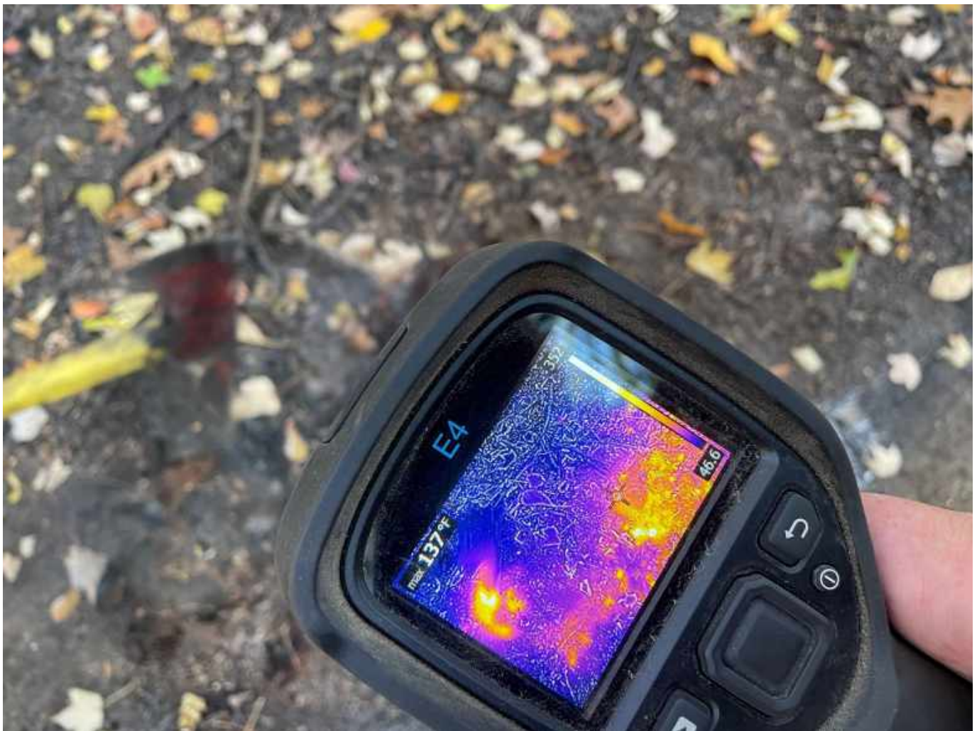
Figure 1: At Willow Metropark, Natural Resources staff utilizes a FLIR infrared camera to detect hotspots within a prescribed fire unit. This tool is able to detect hot areas on and under that ground that might not be visible to the naked eye.
